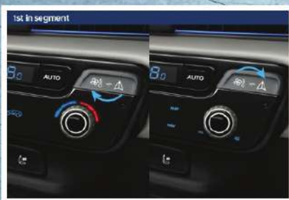
SWITCHABLE TYPE INFOTAINMENT AND CLIMATE CONTROLLER
